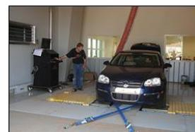
The facility houses a dynamometer for stationary testing of light and medium duty vehicles. This emissions component will further the work of quantifying biofuel carbon footprint.
